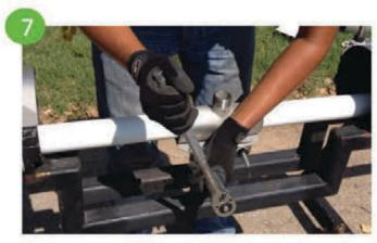
If necessary to reposition, loosen nuts prior to moving saddle and then retorque.
