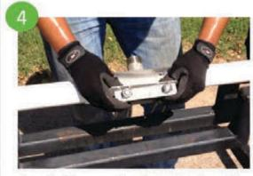
Close lug fingers and studs together by pulling the washer bar upward and snap the lip over the finger base plate. Manually tighten nuts.
